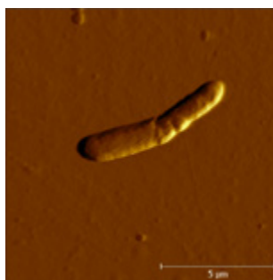
Image of an E Coli cell measured with the Dunk and Scan probe holder.
