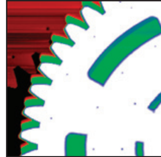
40 x 40 \mu image of a gear fabricated with MEMS.
